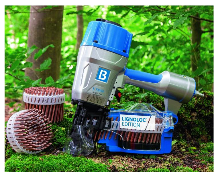
The heat from the penetration process causes a chemo-mechanical reaction between nail and penetrated wood "locking" them together. LignoLoc® nails can be driven into solid structural timber with the Fasco® pneumatic nailer. With the official approval of the DIBt in 2020, Lignoloc® nails are allowed for use in load bearing shear wall constructions.
